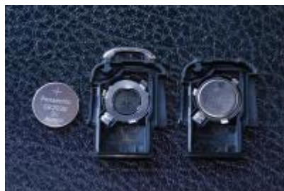
The battery is pretty simple, pop it out. Although I prefer to pry it out with a small jewellers screwdriver as shown.
