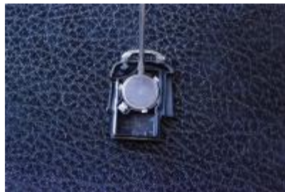
The battery is pretty simple, pop it out. Although I prefer to pry it out with a small jewellers screwdriver as shown.
